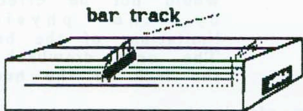
Bar tracks along the top of the strings. Picking and blocking device replaces your right hand.
